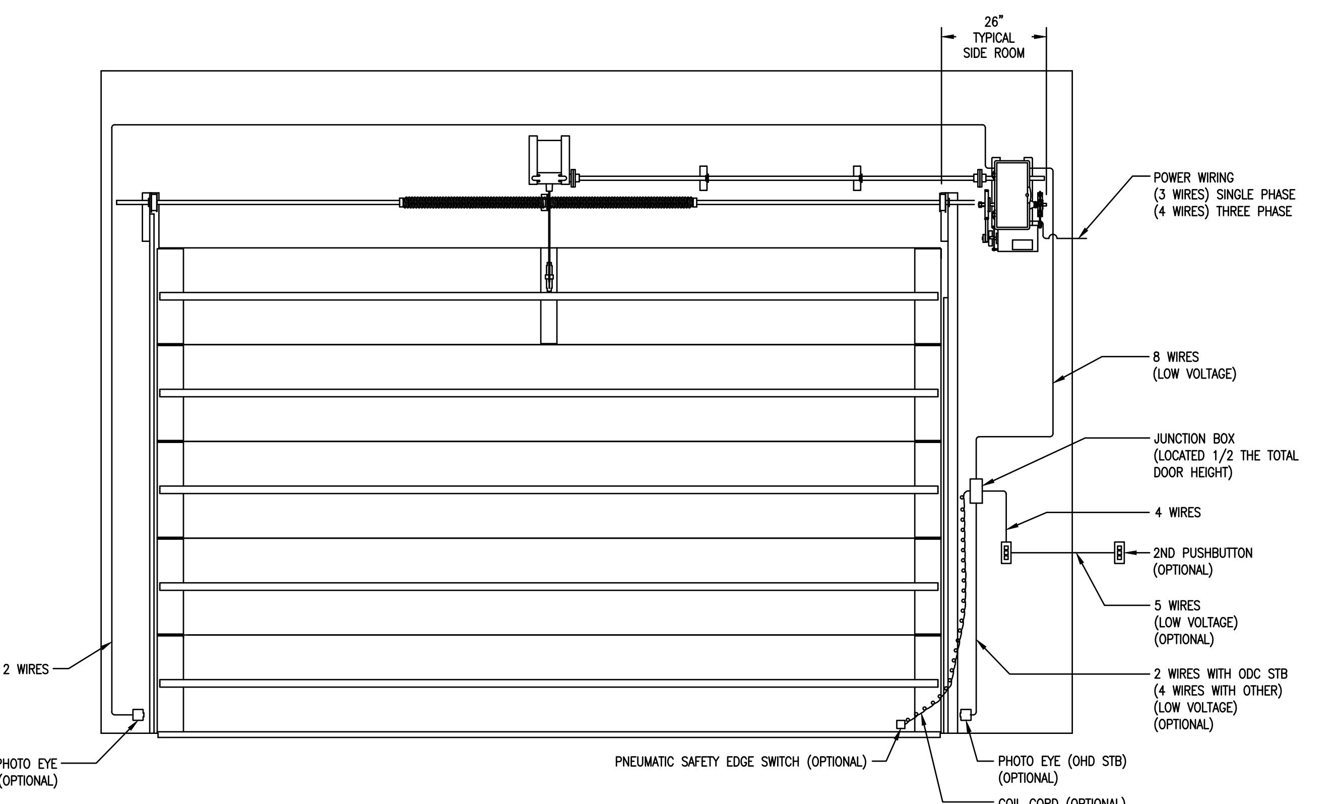
4 TYPICAL OVERHEAD DOOR WIRING DIAGRAM
