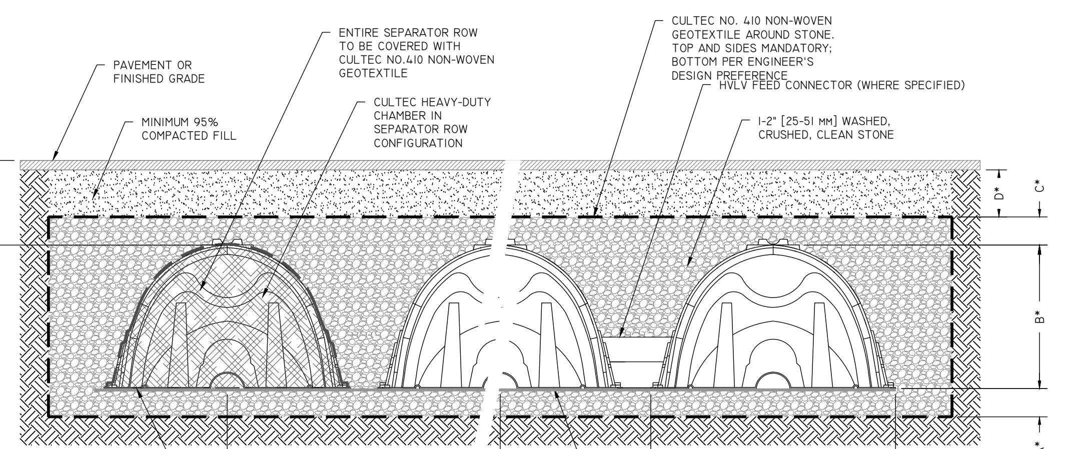
**TYPICAL SEPARATOR ROW CONFIGURATION CROSS SECTION**
