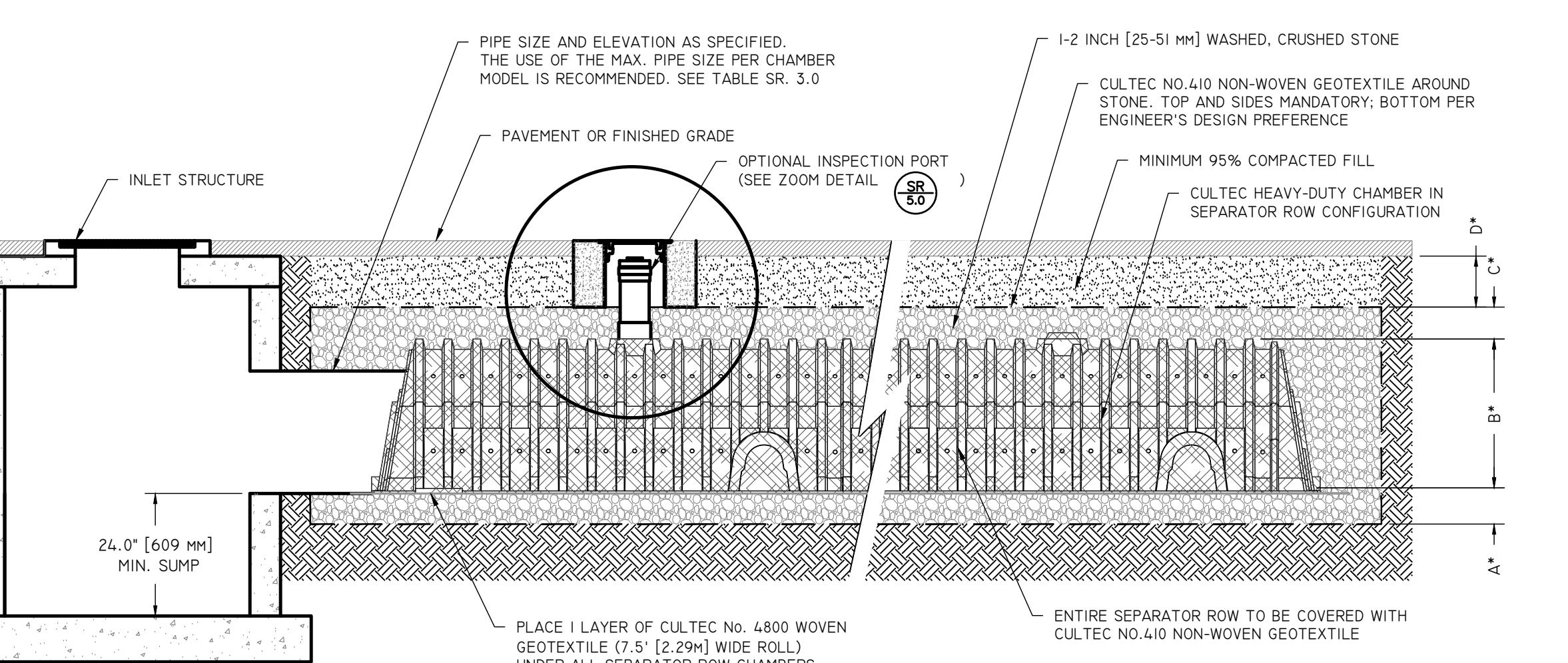
**TYPICAL SEPARATOR ROW CONFIGURATION CROSS SECTION WITH
